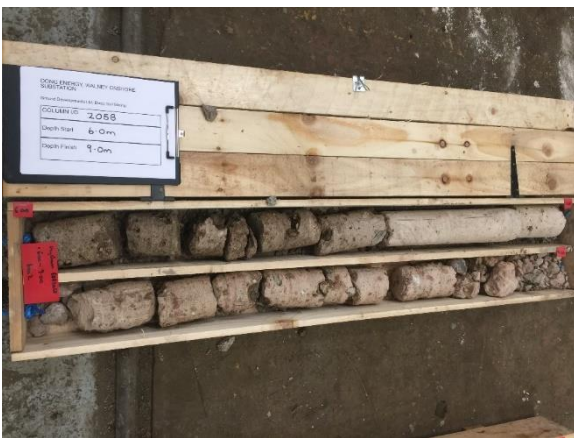
Figure 7. Partial rotary core through soil mix column (courtesy of Ground Developments Ltd)
